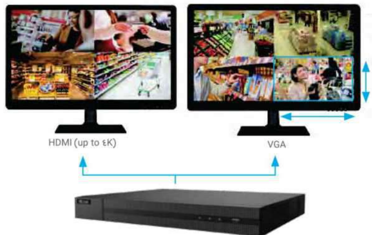
Discrete channel output to two monitors
